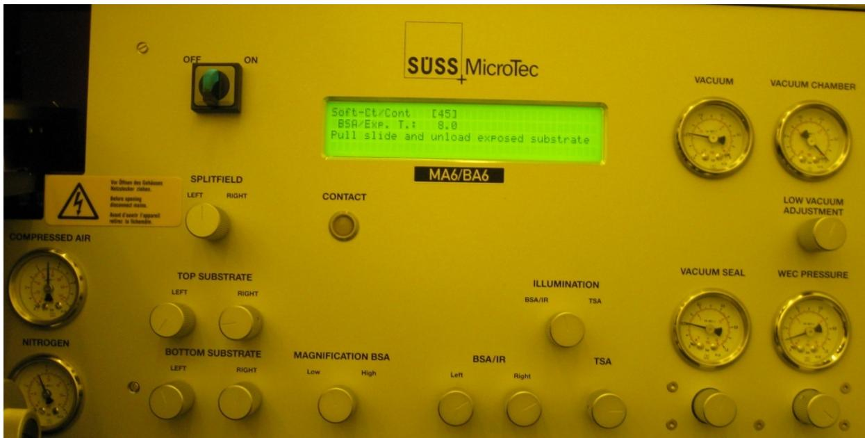
Figure 2: Front panel on MA6
